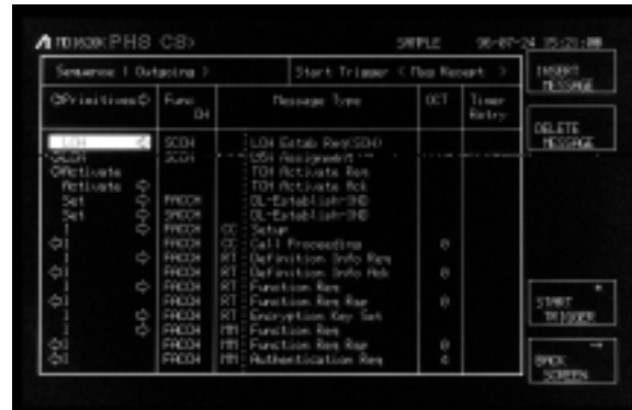
Sequence setting screen (CS simulation mode: origination sequence)
